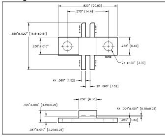
UNLESS OTHERWISE NOTED, TOLERANCES ARE INCHES ±.005" [MILLIMETERS ±0.13mm]
