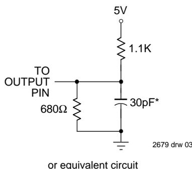
Figure 1. Output Load
