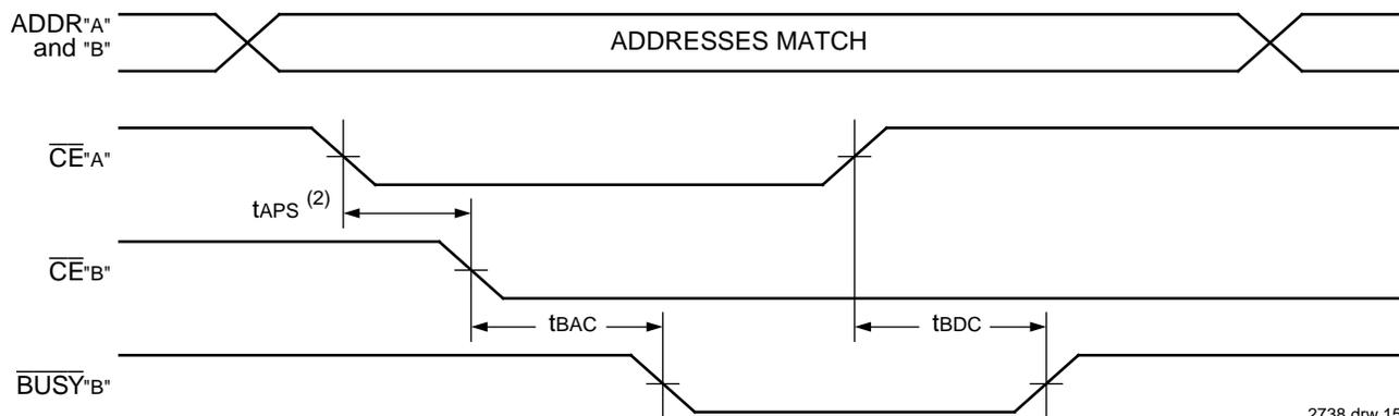
**WAVEFORM OF BUSY ARBITRATION CYCLE CONTROLLED BY ADDRESS MATCH TIMING ( $M/\overline{S} = V_{IH}$ )<sup>(1)</sup>**
