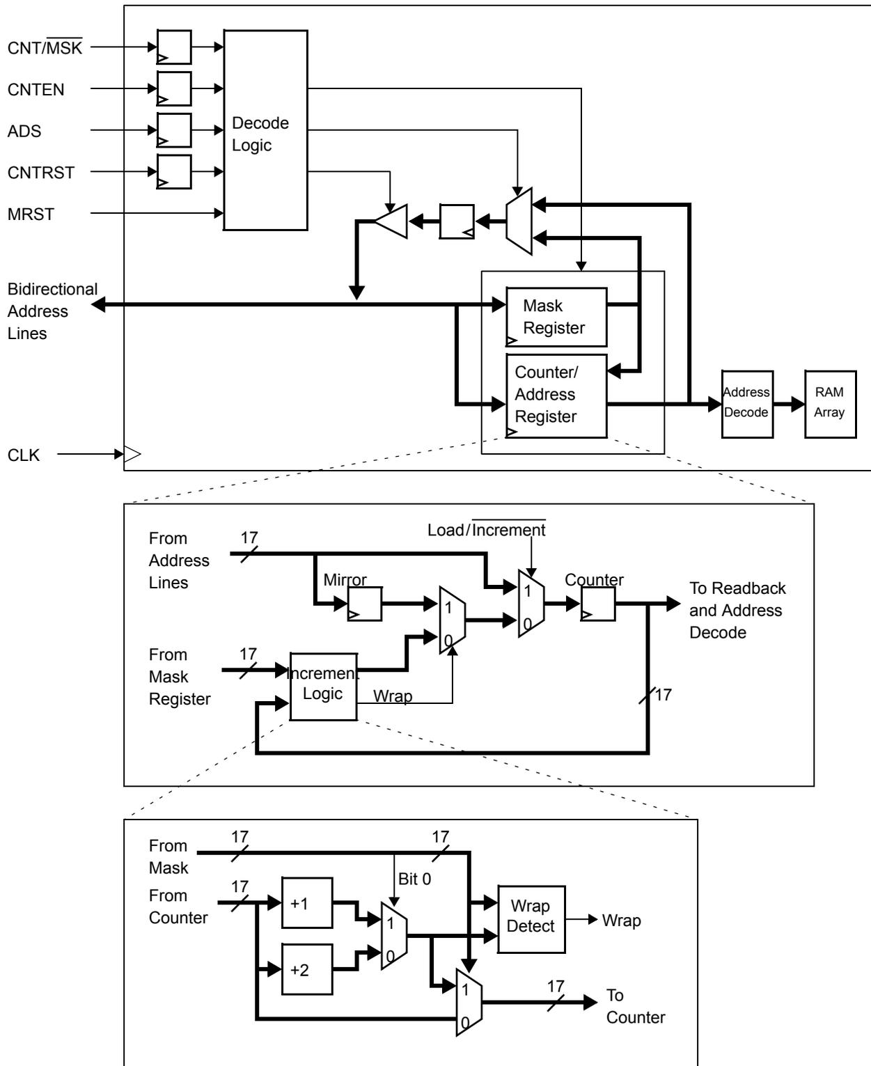
Figure 1. Counter, Mask, and Mirror Logic Block Diagram<sup>[1]</sup>
