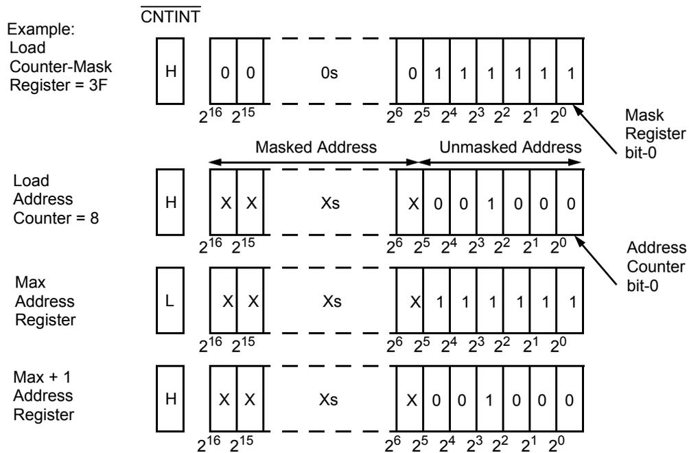
**Figure 2. Programmable Counter-Mask Register Operation<sup>[1, 12]</sup>**
